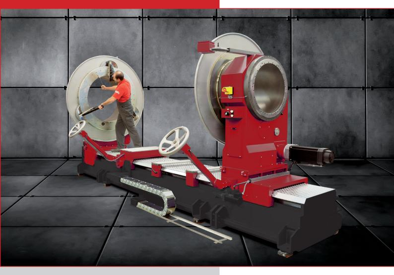
Machine series SYPF especially excels by its sophisticated design, modern and solid construction at operational reliability and highest precision. It was designed for processing particular large diameter tubes and it is mainly used in the quartz glass semiconductor industry.
